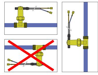
The 315 series flow switch can be installed on either vertical or horizontal piping, but not upside down.
