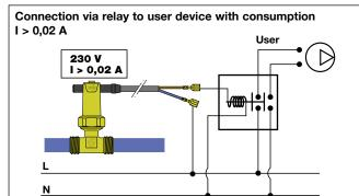
**N.B.**: It is recommended to pay attention to the current consumption value of the user device the flow switch is connected to. If this value is greater than **0,02 A**, a relay must be installed between the flow switch and the user device itself to prevent damage to the flow switch contacts.
